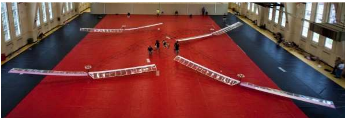
Figure 4.14: UMD Human powered helicopter in flight, summer 2011
